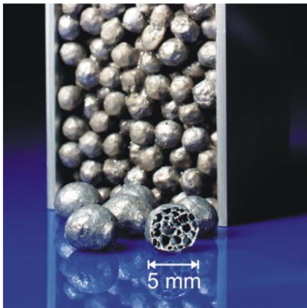
Fig. 7 Opened extrusion profile with APM aluminium foam–polymer hybrid filling (front: single foam elements including cross sectional view)
