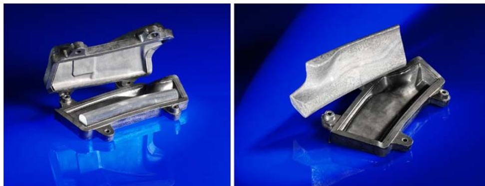
Fig. 3 Near-net shape aluminium foam part production by expansion of foamable precursor material in temperature resistant foaming moulds, e.g., made of cast iron (left: precursor rod in open mould; right: finished aluminium foam part and bottom mould halve)
